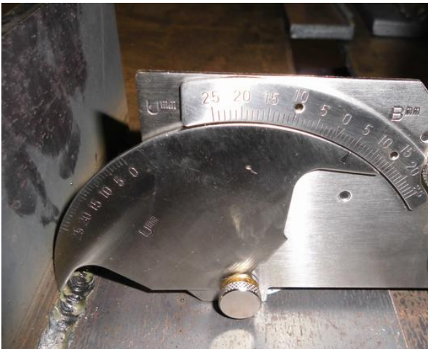
Fig.11 Confirmation of weld leg length
