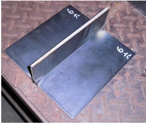
Fig.6 Welding specimen
