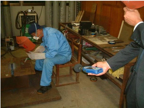
Fig.10 Measurement of welding arc sound
