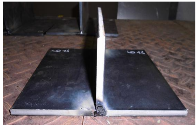
Fig.8 Temporary weld joint
