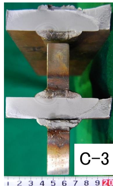
Fig.4.14 Fracture surface after fatigue test
