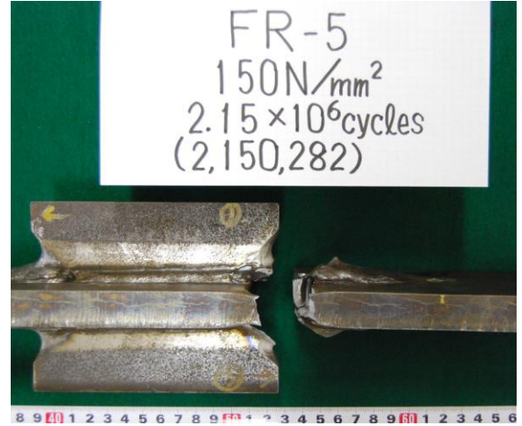
Fig.4.30 Fracture pass after fatigue test
