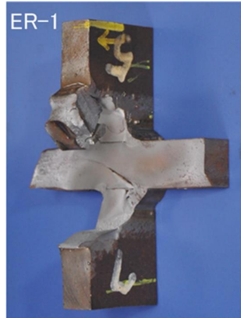
Fig.4.26 Fracture pass after fatigue test
