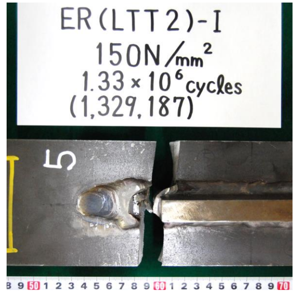
Fig.4.39 Fracture pass after fatigue test
