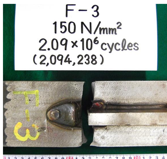
Fig.4.21 Fracture pass after fatigue test
