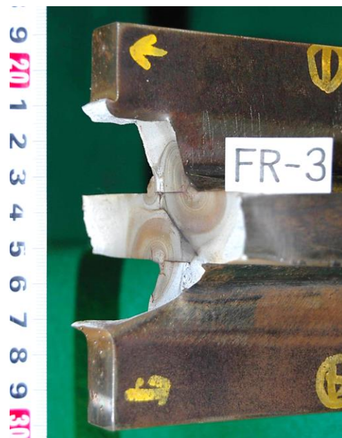
Fig.4.34 Fracture pass after fatigue test
