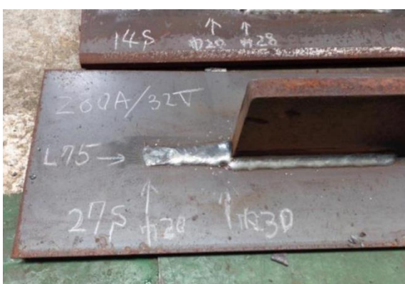
Elongated Bead (L: 75mm, W: 20~30mm)
