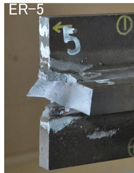
Fig.4.28 Fracture pass after fatigue test
