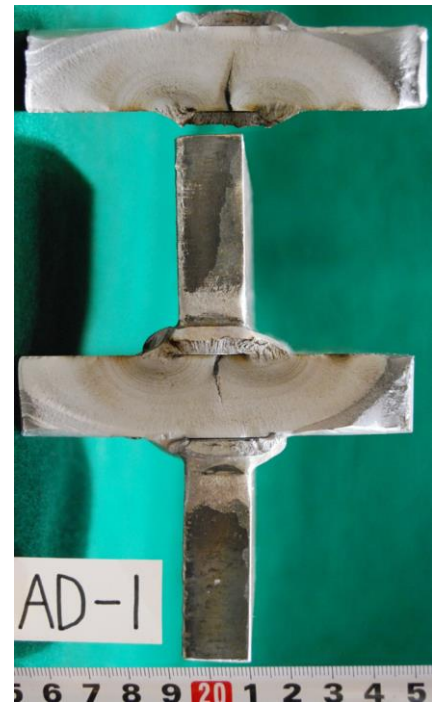
Fig.4.8 Fracture surface after fatigue test
