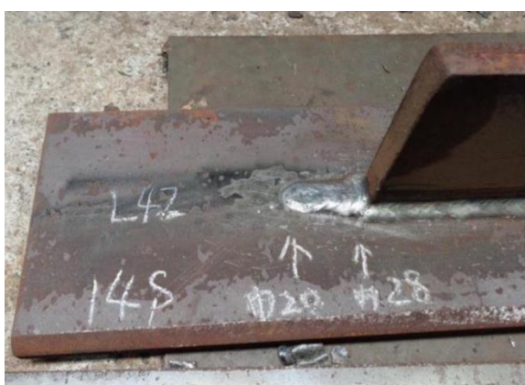
Elongated Bead (L: 42mm, W: 20~28mm)
