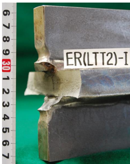
Fig.4.40 Fracture pass after fatigue test
