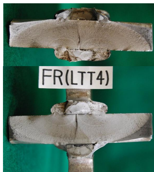
Fig.4.45 Fracture pass after fatigue test
