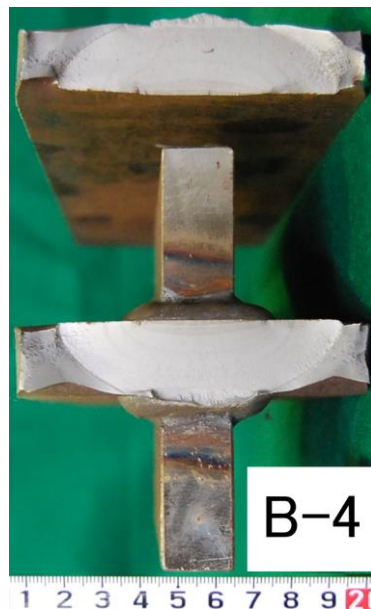
Fig.4.13 Fracture surface after fatigue test
