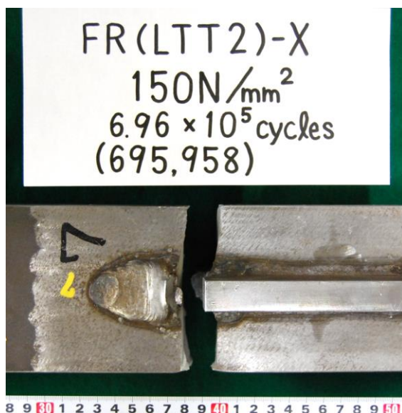
Fig.4.42 Fracture pass after fatigue test
