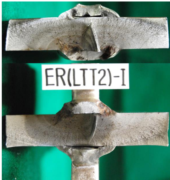
Fig.4.38 Fracture surface after fatigue test
