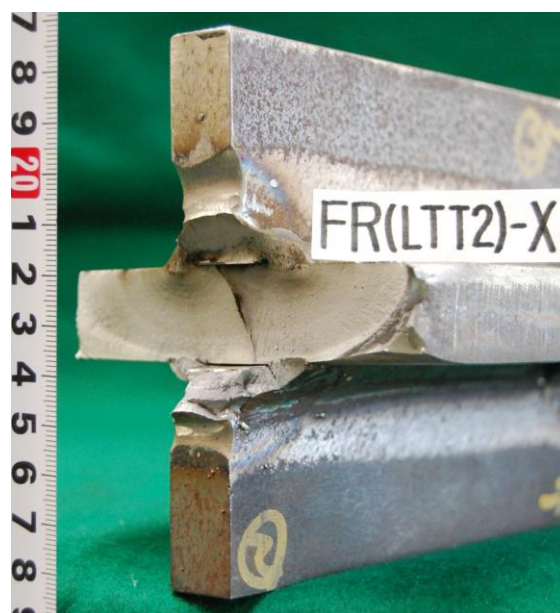
Fig.4.43 Fracture pass after fatigue test
