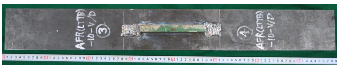
[Vertical Downward Position : AFR(LTTB)-10-V/D]
