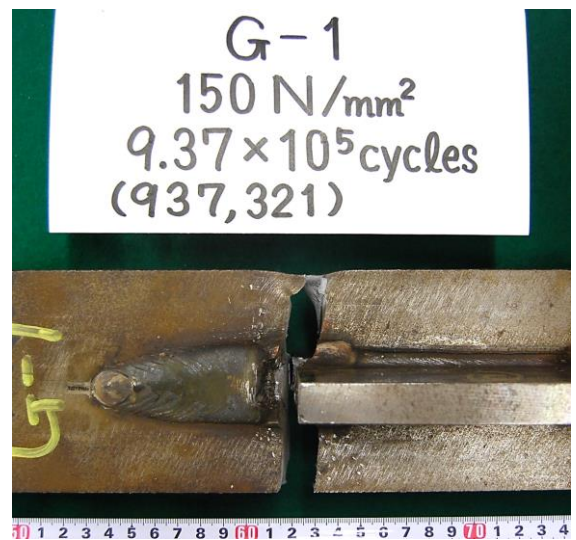
Fig.4.23 Fracture pass after fatigue test
