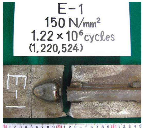
Fig.4.16 Fracture pass after fatigue test
