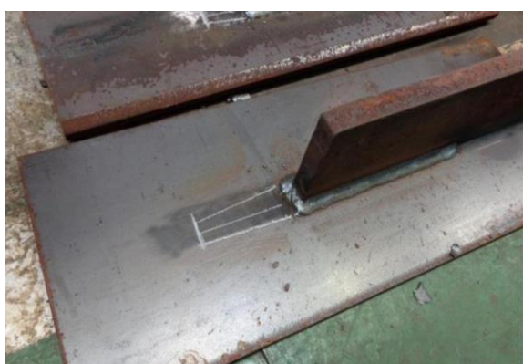
Marking (Elongated Bead: 75mm)
