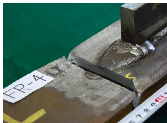
Fig.4.36 View of boxing fillet welded joint toe
