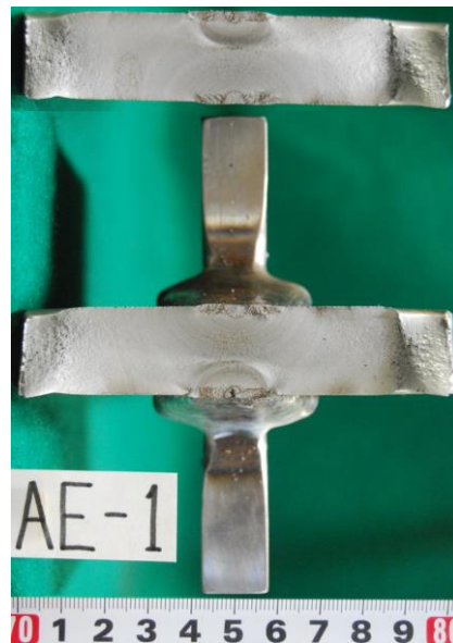
Fig.4.9 Fracture surface after fatigue test
